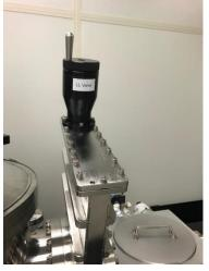
3.2.8. Align the black sharpie mark on the platen rotation motor coupling with the window as shown.
