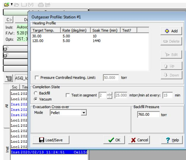
Click on Load in the menu for that station. If loading both stations, they can both be inserted and the Load All in the ALL submenu selected. The instrument will first equalize the pressure in the manifold with the sample pressure to avoid elutriation of the sample and then evacuate the sample. When the crossover pressure is reached, and the course vacuum is opened, the heating profile loaded will begin.
