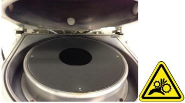
3.8 Click "Utilities"/"Pump Chamber (Turbo)" and using one hand, push down on the chamber handle. Continue to push down until the "Roughing" valve opens. You will be able to hear the chamber pump down. The lid has new air lift cylinders. This problem should go away eventually.
