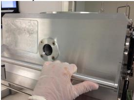
It will take several minutes to pump down all the way. Do not continue until the pressure toggles between 0 mTorr as displayed below.
