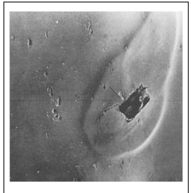
Fig. 49. The two black lines (center) are burnt traces of line scan.
