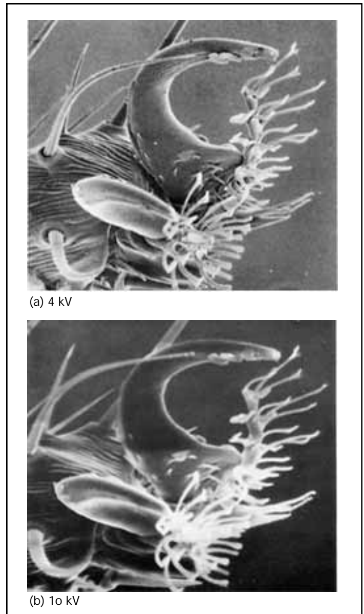
Fig. 22. Specimen: Fbreleg of vinegar fly. Charge-up can be reduced by using low accelerating voltage.
